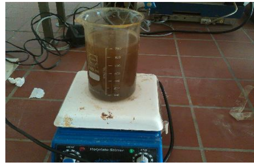
Fig. 3. Diatomite modified by iron (DMF4) during stirring Fig. 4. Iron-modified diatomite (DMF4) after agitation and oxidation by air
